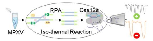
CRISPR is combined with nanopore sensing technology to detect whether or not mpox is present in a sample.
